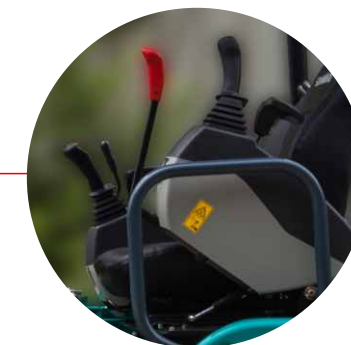
Safety switch of pilot control
